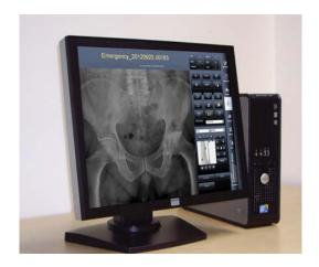
High definition images are captured with the Varian 17in x 17in , 9 megapixel, cesium flat panel detector. Images are then displayed in seconds on the Barco 19in TFT, color LCD clinical review display. This 1280 x 1024 resolution display with touch screen interface is DICOM compliant providing more accurate grayscales and better contrast than standard monitors.
